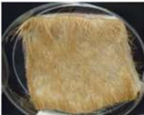
Figure 6. The piece of cow's skin after immersion in crude alkaline enzyme extract for 150 min.
