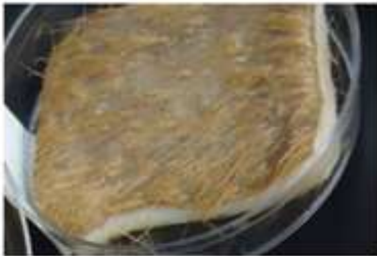
Figure 5. The piece of cow's skin after immersion in crude alkaline enzyme extract for 120 min.
