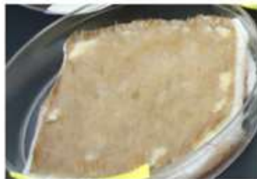
Figure 3. The piece of cow's skin after immersion in crude alkaline enzyme extract for 60 min.
