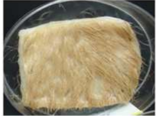
Figure 7. The pieces of cow's skin immersion by crude alkaline enzyme after 180 min.
