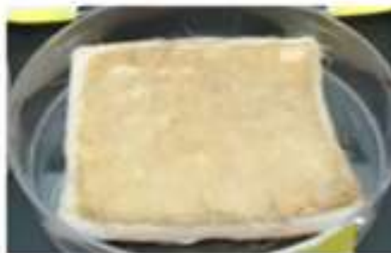
Figure 2. The piece of cow's skin after immersion in crude alkaline enzyme extract for 30 min.
